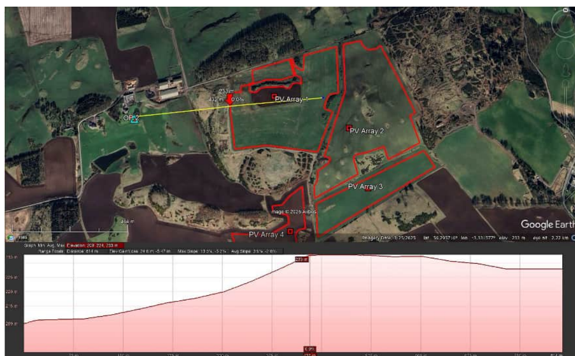
Graphic 5-4: Elevation profile between OP 2 and PV Array 1 where glare emanates.
