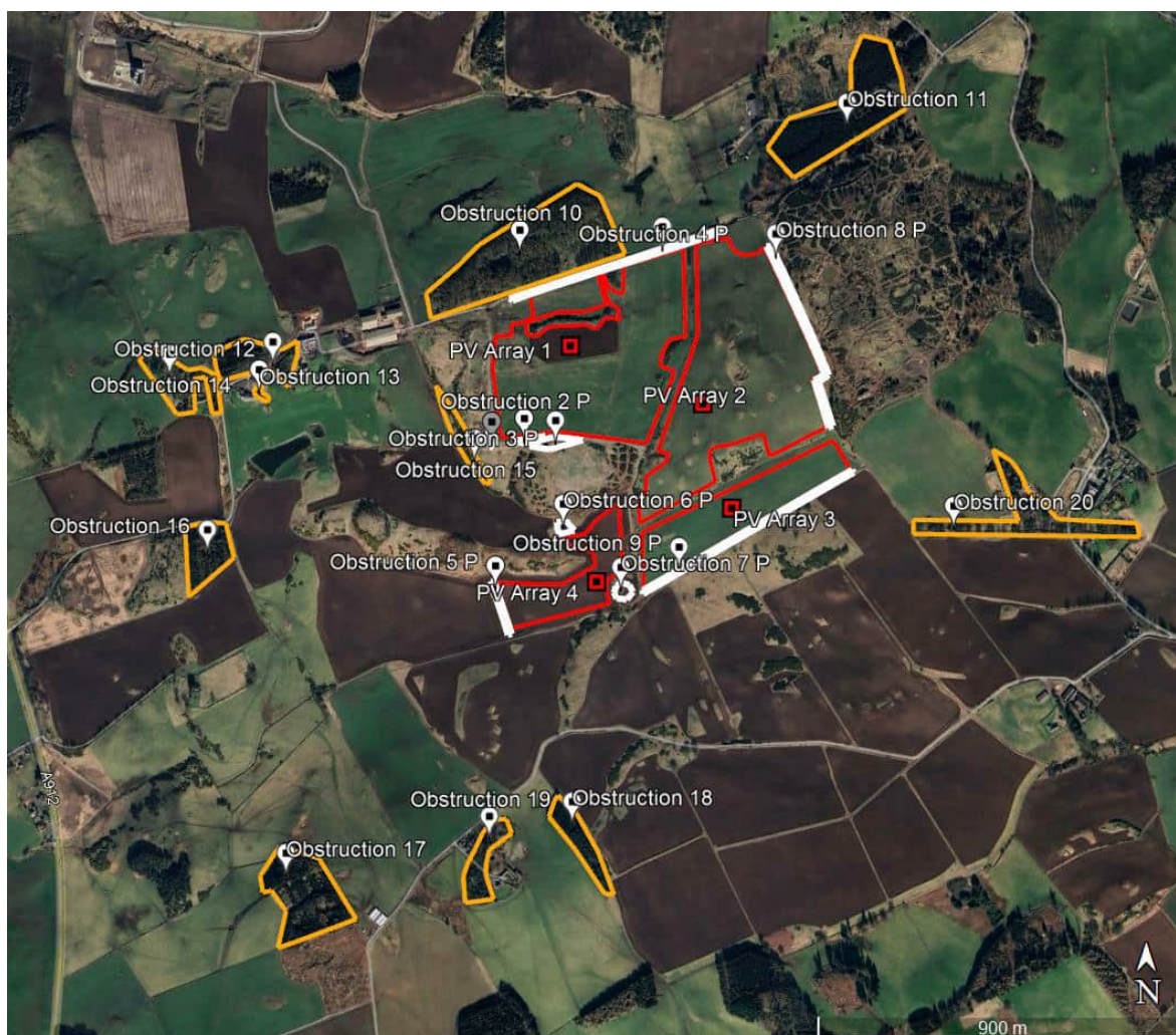
Graphic 5-1: Existing (orange) and proposed screenings (white) included in the simulation.
